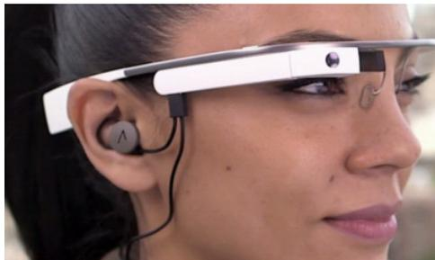
Glass is a wearable computer being developed by Google. At first glance Glass appears to be no more than a pair of designer glasses. However, the system works like a hands-free smartphone that displays visual information on the lens of the Glass. The technology is voice-operated and is also linked to the internet. It is not currently available outside the USA. For more information go to a review of Google Glass :
